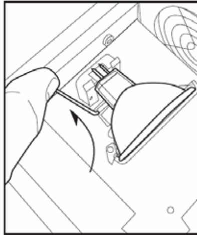
STEP 2 Push down lever to release the lamp from its bracket.
