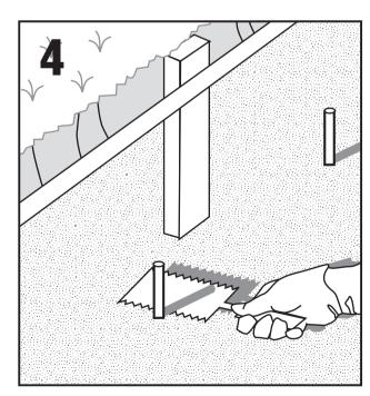
**STEP 4:** When the concrete has set, cut the light stick flush at the concrete surface with a saw or a grinder. Use a sander to produce a smooth finish on the light stick.
