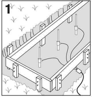
**STEP 1:** Place light sticks firmly into the ground with the fiber optics attached and the coupler assembled. The top of the light stick should extend 2" above the final concrete grade.
