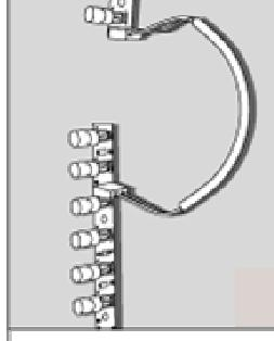
Jumper cables can be connected to any available socket on the Flex-LED Strip.
