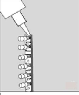
Apply a small amount of dielectric grease to the pin socket receptacle prior to installing the jumper cable connector, or another option is, after installing jumper cables apply silicone over entire connector plug. Note: All connectors used and unused must be sealed with silicon or dielectric grease to prevent corrosion.
