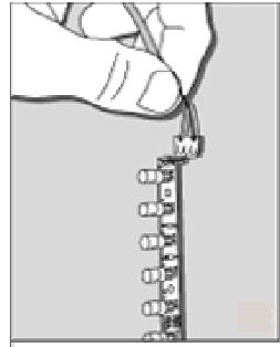
Snap jumper cable connector plug into pin socket receptacle by pushing firmly into socket.
