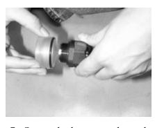
7. Screw the lens over the end of the fiber tight connector until the o-ring makes a tight seal.
