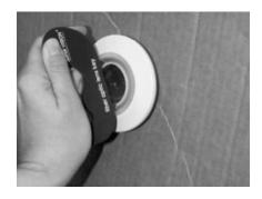
10. Tighten the retaining ring snug.
