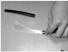
2. Inspect the fiber for any damage. Re-cut if necessary.
