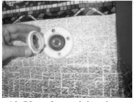
10. Place the retaining ring over the lens and turn clockwise to tighten. Make sure the two rubber gaskets are in place before you install the retaining ring.
