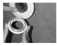
9. Place the retaining ring over the lens and turn clockwise to tighten. with the lens wrench until it is
