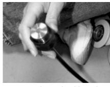
3. Insert the proper reducer fitting. The fiber should be tight inside of the reducer.
