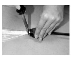
5. With a pre-heated hot knife, cut the fibers across the reducer. Do NOT use a sawing motion. Let the heat of the blade cut the fiber.
